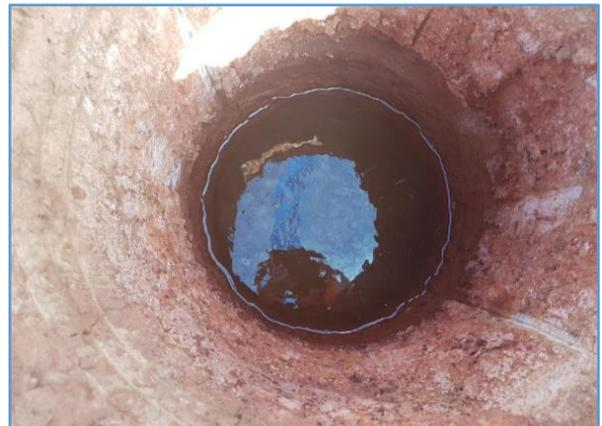
*Test borehole water level depth - 0.47mtr (15<sup>th</sup> May)*
