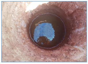
Test borehole water level depth - 0.47mtr (15th May)
